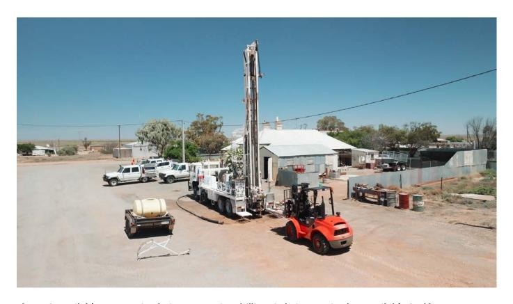
**Figure 2** Havilah's reverse circulation percussion drilling rig being serviced at Havilah's Cockburn exploration base-camp prior to being mobilised to the first of its planned 2023 drilling sites last week.
